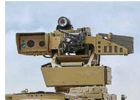
Remote Controlled Weapon Station FLW 200, ready for three different calibers of machine guns
