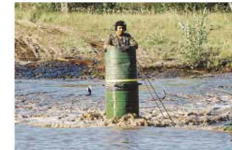
LEOPARD 2 in submerged operation for crossing water obstacle
